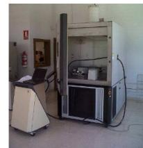
The testing equipment for waterproofing used are the following: Pressure Equipment, IPT Airless Basic Climatic Chamber Thermotron with certified calibration 10/34513341 of the 20-9-2010 Pattern Measure of Pressure: Telegan Pressure Transducer XMLP010BC71V certified 12/34508029 of the 27-3-2012
